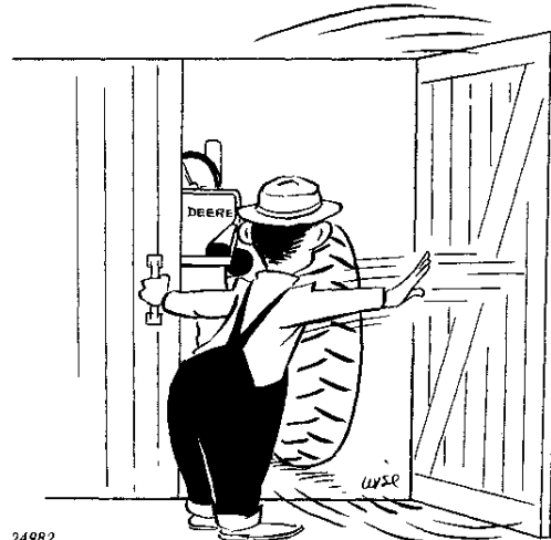
Always Make Sure There Is Plenty of Ventilation Before Starting the Engine
